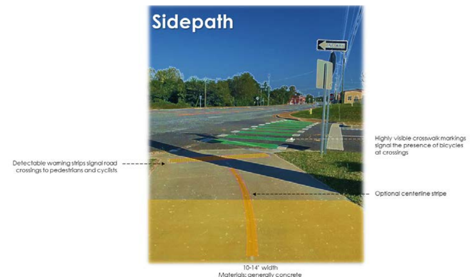
Figure 41. Sidepath Typical Sections
